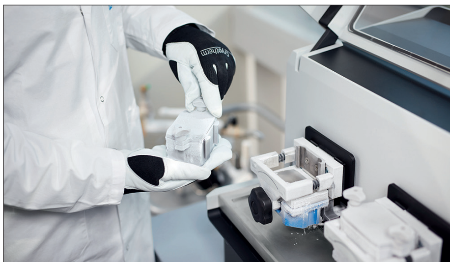
Figure 2: Cooling concept based on thermal plates: the sample material is processed in Screw Lock Jars which are mounted on top of the thermal plates.
