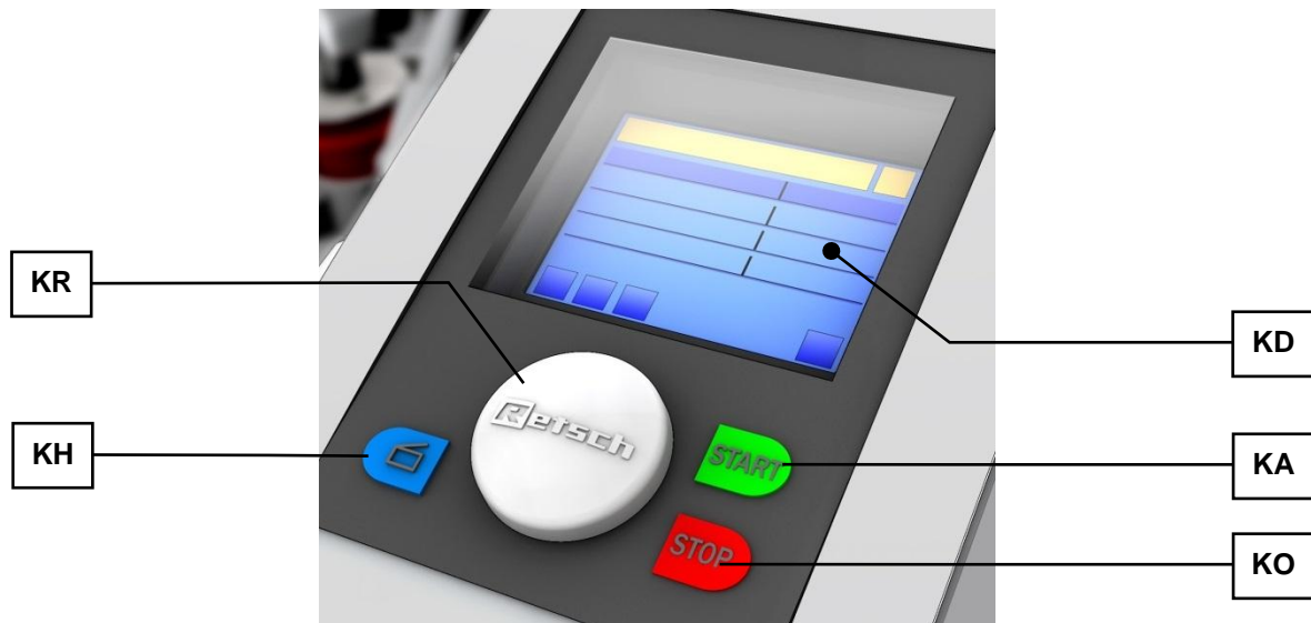
Fig. 11: View of the control panel
