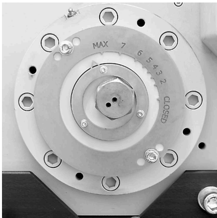
Scale for continuous gap width setting
