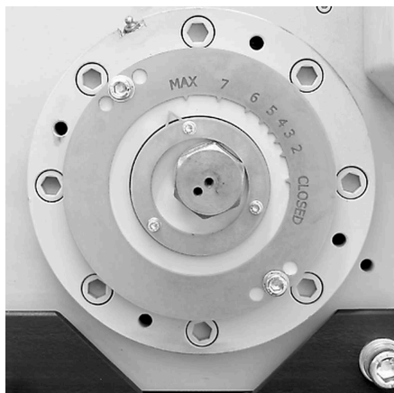
Scale for continuous gap width setting
