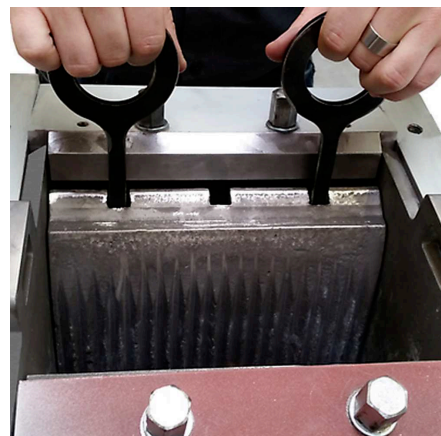
Jaws and wearing plates can be replaced
