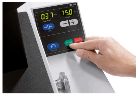
Digital speed setting and display of gap width
