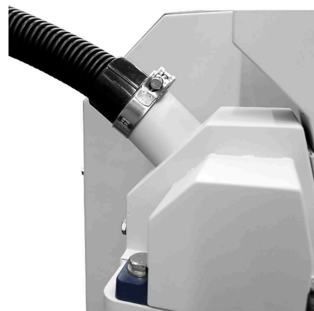
Connection for dust extraction
