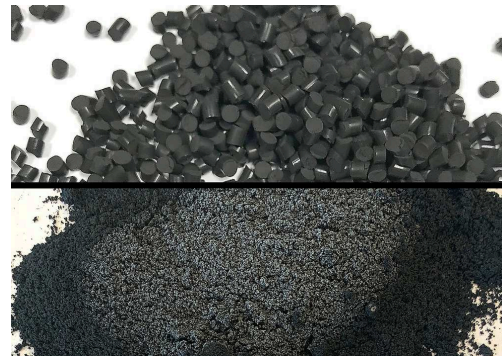
Fast milling of black Fluoro-carbon rubber (FKM) by embrittling the sample in two 125 ml jars at -100 °C.
