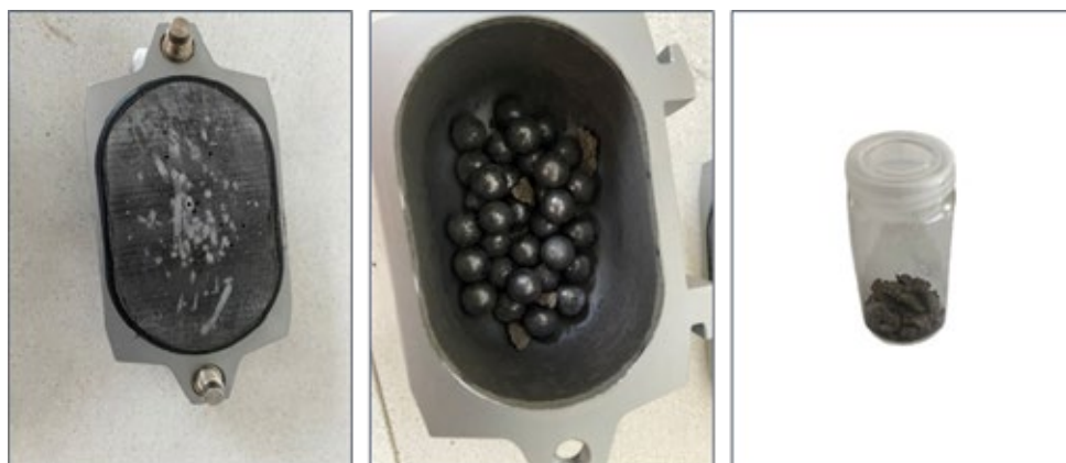
Figure 1: Pictures of the lid (left), the jar (middle), and the compound after the milling (right)
