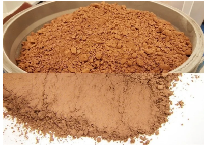
3 kg Iron ore in RS 300 in 12 min, < 100 \mu\text{m} . Image Credit: RETSCH
