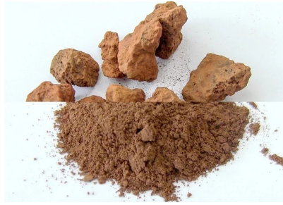
120 g Iron ore in RS 200 in 1 min, < 100 \mu\text{m} . Image Credit: RETSCH
