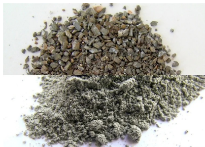
10 g Ore in MM 400 in 2 min, < 100 \mu m. Image Credit: RETSCH
