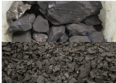
20 kg Mangan ore in BB 300 with a gap of 10 mm and 1 mm in 3 min. Image Credit: RETSCH
