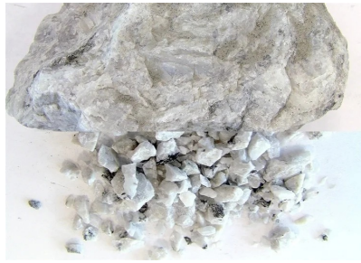
10 kg Diorite in BB 300 with a gap of 1 mm in 1.5 min. Image Credit: RETSCH
