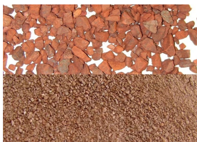
200 g Iron ore in BB 50 with a gap of 0.1 mm in 1 min. Image Credit: RETSCH
