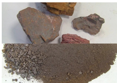
200 kg/h in BB 500 with a gap of 0.1 mm in 2.5 min. Image Credit: RETSCH
