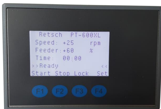
Fig. 23: Locked and ready to start
