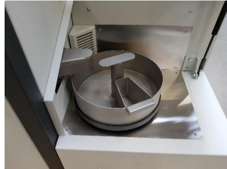
Fig. 19: Inserted part module for 8 part samples or one part sample with rejection mechanism
