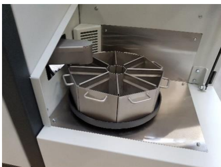
Fig. 19: Inserted part module for 8 part samples or one part sample with rejection mechanism
