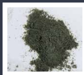
❸ PULVERIZATION IN THE CRYOMILL TO 200 µm
