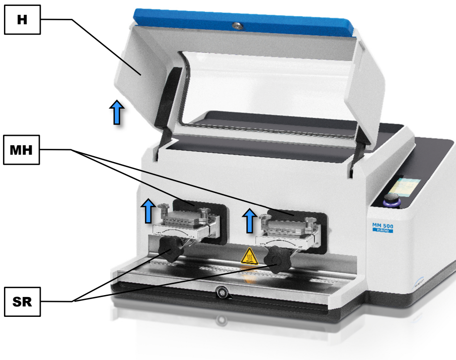
Fig. 30: Removing the sample material
